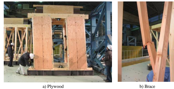
Fig. 5 Damages on the specimens in the JMA Kobe
